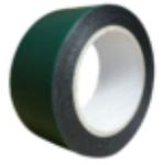
volzMount V5331 is a double-sided, closed-cell, medium density, PE-foam coated with a high-performance acrylic adhesive, protected by a siliconized PE-release liner. Designed for glazing applications, mounting and assembling of body side mouldings, emblems, mirrors, labels, etc. Plastic liner for easy removal.
