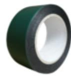
volzMount V5331 is a double-sided, closed-cell, medium density, PE-foam coated with a high-performance acrylic adhesive, protected by a siliconized PE-release liner. Designed for glazing applications, mounting and assembling of body side mouldings, emblems, mirrors, labels, etc. Plastic liner for easy removal.
