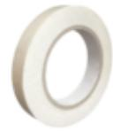
volzMount V5321 is a double-sided, self-adhesive tape with a 70 kg/m<sup>3</sup>, closed-cell, PE-foam carrier and a clear, solvent-acrylic adhesive. It has a very aggressive adhesive, high tack, good cohesion, and a high holding power at high and low temperatures.
