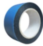
volzMount V5320 is a double-sided, 0,8 mm black, closed cells, medium density PE foam coated with a high performance acrylic adhesive system and protected by siliconized PP release liner. Designed for glazing applications, mounting and assembling of body side mouldings, emblems, mirrors, labels, etc. Plastic liner for easy removal.
