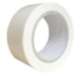
volzMount V5312 is a double-sided, self-adhesive tape with a closed-cell, medium density PE-foam carrier and a high-performance, acrylic adhesive. It has a high initial tack and shear strength, excellent UV and aging resistance, and it adheres well to a variety of smooth and rough surfaces. volzMount V5312 is designed for general mounting and assembling applications in the automotive, furniture, building and construction industries.
