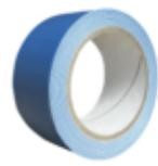
volzMount V5311 is a double-sided, self-adhesive tape with a 95 kg/m<sup>3</sup>, closed-cell, PE-foam carrier and a clear, solvent-acrylic adhesive. It has a very aggressive adhesive, high tack, good cohesion, and a high holding power.
