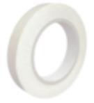
volzMount V5306 is a 0,5 mm white, closed cells, high density PE foam coated with a high performance acrylic adhesive system and protected by siliconized paper release liner. Designed for mounting and assembling displays, emblems, decorative profiles, nameplates, etc. Ideal for all applications where high shear strength and UV resistance are required.
