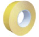
volzMount V4300 PV1 is a double-sided, self-adhesive tape with a 75 kg/m<sup>3</sup>, closed-cell, PE-foam carrier and a white, synthetic-rubber adhesive. It has a very aggressive adhesive, high tack, good cohesion, and a high holding power at high and low temperatures.
