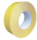
volzMount V4300 PV1 is a double-sided, self-adhesive tape with a 75 kg/m<sup>3</sup>, closed-cell, PE-foam carrier and a white, synthetic-rubber adhesive. It has a very aggressive adhesive, high tack, good cohesion, and a high holding power at high and low temperatures.
