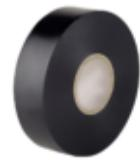
volzFlex 1086 PV5 is a 0.18 mm thick, professional, self-extinguishing, electrically insulating soft PVC adhesive tape in premium quality with an aggressive, pressure-sensitive rubber-based adhesive. The tape complies with REACH and the European Directive 2011/65/EC (RoHS 2) and the Commission Delegated Directive (EU) 2015/863 (RoHS 3).
