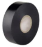
volzFlex 1086 PV5 is a 0.18 mm thick, professional, self-extinguishing, electrically insulating soft PVC adhesive tape in premium quality with an aggressive, pressure-sensitive rubber-based adhesive. The tape complies with REACH and the European Directive 2011/65/EC (RoHS 2) and the Commission Delegated Directive (EU) 2015/863 (RoHS 3).
