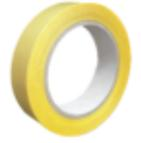
volzFix V6171 PV1 is a double-sided self-adhesive tape consisting of a paper Non-Woven carrier, layered on both sides with a modified, solvent free dispersion acrylate adhesive. This powerful adhesive has high temperature, aging, and plasticiser resistance. It is lined with a double-sided silicone paper.
