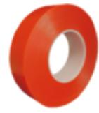
volzFixV5133 PV2 is a double-sided adhesive tape consisting of a polyester film backing coated on both sides with a modified acrylic adhesive. It features high resistance to UV radiation, temperature effects, chemicals and solvents, and moisture. In addition, the tape is suitable for permanent bonding to low-energy metal and paint, as well as high-energy plastic surfaces.
