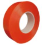
volzV5133 PV1 is a double-sided adhesive tape consisting of a polyester film backing coated on both sides with a modified solvent acrylic, pressure-sensitive adhesive. It features high resistance to UV radiation, temperature effects, chemicals and solvents, and moisture. In addition, the tape is suitable for permanent bonding to low-energy metal and paint, as well as high-energy plastic surfaces.
