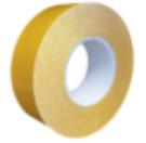
volzFix V4125 is a double-sided, self-adhesive tape produced of a clear BOPP-film carrier and a white, hot-melt, synthetic-rubber adhesive. The product is perfect for carpet laying or bonding of metal and plastics where no high temperatures is needed. The product also has a very high tack.
