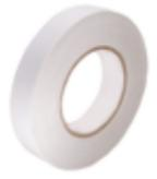
volzFix 9086 is a double-sided, self-adhesive tape consisting of a Non-Woven carrier and a modified-solvent, acrylic adhesive. It is characterized by a very good adhesion and very high temperature resistance and is also suitable for difficult applications. The tape has a good UV resistance and is compatible with other materials.
