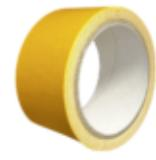
volzFix 9064V is a tear-resistant tape coated on both sides, consisting of a cloth carrier and a rubber adhesive. It can be used universally and is suitable for bonding rough surfaces and can be removed without residue.
