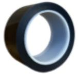
volzElektro 6215 PV4 is manufactured from 50-micron polyester film coated on one side with a high-quality silicone adhesive system. Designed for masking in high temperature applications where a strong backing combined with an excellent chemical resistant adhesive is required.
