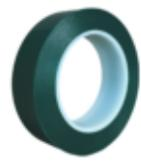
volzElektro 6215 PV3 is a 2 mils polyester (PET) film with 1,20 mil highly efficient, silicone adhesive. This product was designed to provide high tack and adhesion, and has a strong resistance to corrosive chemicals. It can be easily removed from applied surface without adhesive residue, making it an excellent tape for masking applications and to be used for powder coating.
