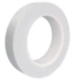
volzElektro 6018 PV4 consists of a highly tear-resistant glass fabric backing coated with a thermosetting silicone adhesive. The tape is flame retardant and therefore UL 510 listed. It is suitable for use at high continuous temperatures of up to 200°C..
