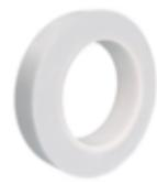
volzElektro 6018 PV4 consists of a highly tear-resistant glass fabric backing coated with a thermosetting silicone adhesive. The tape is flame retardant and therefore UL 510 listed. It is suitable for use at high continuous temperatures of up to 200°C..
