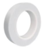
volzElektro 6018 PV3 consists of a highly, tear-resistant, glass fabric backing coated with a thermosetting, silicone adhesive. The adhesive tape is flame retardant and is UL 510 listed. It is suitable for use at high continuous temperatures of up to 200°C.
