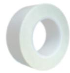
volzElektro 6017 PV4 is a glass cloth electrical tape manufactured from an electrical grade fiberglass cloth with high performance thermosetting acrylic adhesive. The tape has excellent resistance to solvent and flagging. For covering uses in coil, layer and wire harness applications. Insulating function for crossover and other component as well.
