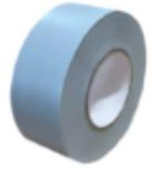
volzElektro 5017 is a self-amalgamating insulating adhesive tape made of silicone rubber. Suitable for protecting and repairing medium-voltage cable terminations, and as a protective layer against flowing oil and grease for impregnated cable connections. volzElektro 5017 can also be used for a variety of household repairs, e.g. broken pipes, handles, repairing frayed ropes and much more.
