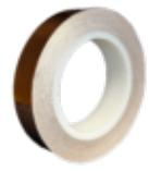
volzElektro 4384 PV1 consists of high tear-resistant copper film, laminated with a acrylic adhesive filled with silver particles. It provides a high conductivity. The adhesive tape has a silicone paper liner. volzElektro 4384 PV1 is solderable and is very good for a variety of applications in EMY / ESD.
