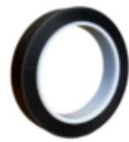
volzElektro 11202 PV3 is a high quality Teflon® electrical insulation tape manufactured from high-modulus, PTFE film with a silicone adhesive. The 2 mils thick backing grants a high breakdown voltage. It is coupled with an outstanding thermal rating and conformability. For uses in coil, capacitor and wire harness insulation at high temperatures. UL recognized flame retardation.
