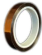
volzElektro 1018 is a Kapton® Polyimide Silicon Adhesive Tape manufactured of a 25µm Kapton® polyimide film single coated with a cured silicone adhesive system, 60µm total thickness. Recommended for a variety of high temperature protection and insulation applications (180°C thermal class H).
