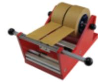
volzDispenser 161-6080 is a special manual bench dispenser for processing adhesive tapes. The product can be fixed on tables or other objects. The desired length will be placed on the cutting bar and by moving the smooth blade to the side, the tape is cut off. The dispenser can take one wide or two narrow rolls. The blade can be exchanged or fastened with the supplied tool.
