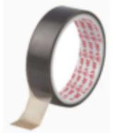
Saint-Gobain / h-old® TF50 is a PTFE (polytetrafluoroethylene) film coated with a high-temperature silicone adhesive system. Designed for high temperature insulation, release wrap on rollers in numerous industries, cure process of composites materials and all applications where a low-friction, anti-stick and non-toxic properties are required. Flame retardant (UL 510)
