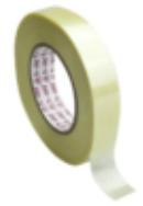
Saint-Gobain / h-old® PR30 is a glass filament reinforced PET film coated on one side with a rubber thermosetting adhesive system. Designed for holding applications where a high tensile strength with a good thermal resistance are required.
