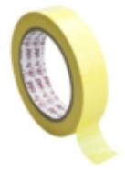
Saint-Gobain / h-old® P315 is PET Film coated on one side with thermosetting rubber adhesive. Designed for coil wrapping, interlayer insulation of electrical motors and transformers, anchoring, holding, harnessing etc.
