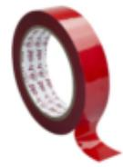
Saint-Gobain / h-old® K50 is a Teonex® film coated on one side with high-temperature silicone adhesive. Designed for high temperature electrical applications where a thin, strong backing combined with excellent dielectrical properties are required.
