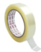
Saint-Gobain / h-old® K30 AC is a Teonex® film coated on one side with high-temperature acrylic adhesive. Designed for high temperature electrical applications where a thin, conformable backing combined with excellent dielectrical properties are required.
