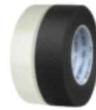
Intertape® 4616 is a glass cloth electrical tape. Woven fibreglass backing imparts high temperature resistance and thermal stability, offering outstanding abrasion resistance for a large number of applications. This tape offers high adhesion and resistance to tearing. The rubber thermosetting adhesive gives the tape excellent solvent resistance.
