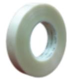
Intertape® 4237 is a PET Film / glass filament reinforced electrical tape. High tensile strength, conformable PET Film coating with an aggressive adhesive for a variety of heavy duty insulating, banding and holding applications. A 1.0 mil PET Film provides puncture, edge tear, and abrasion resistance. This tape is very resistant to chemicals, solvents and aging, and offers high dielectric strength and insulation resistance.
